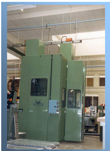
Punch press insulation
